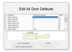
Edit the width of your door stiles and rails. Change the width or height of the panels in multi panel doors, or change the width of your mullions, or the thickness of the bead and more. You can change these dimensions on all the doors or just one door in a job. The parametric changes are reflected in your design and automatically adjust the cut list output for accurate cut sizes.
